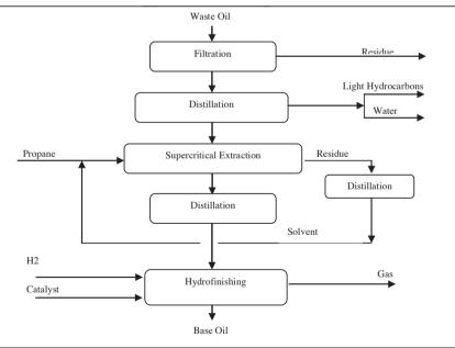
Figure 20 ROSE/Kellog simplified block flow diagram; Source Giovanna et al (2003)
