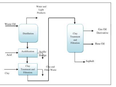
Figure 21 Acid/Clay re-refining process Source: Giovanna et al (2003)
