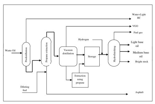
Figure 17 Snamprogetti simplified process flow diagram Source: Snamprogetti
