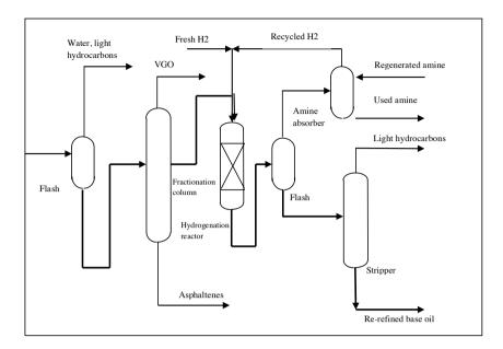
Figure 12 Revivoil simplified process flow diagram Source: Petder (2012)
