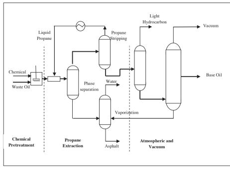
Figure 19 Interline simplified process floe diagram Source: Audibert (2006)
