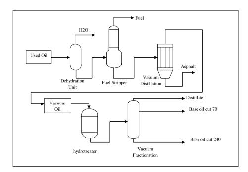
Figure 8 Safety Kleen simplified process flow diagram Source: Fernatt (2013)
