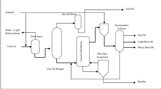
Figure 24 SOTULUB simplified process flow diagram
