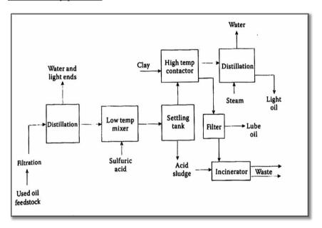
Fig (3) - Acid/Clay Process - Source: 1
