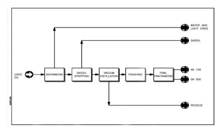
Fig (13) - The STP Process - Source 94
