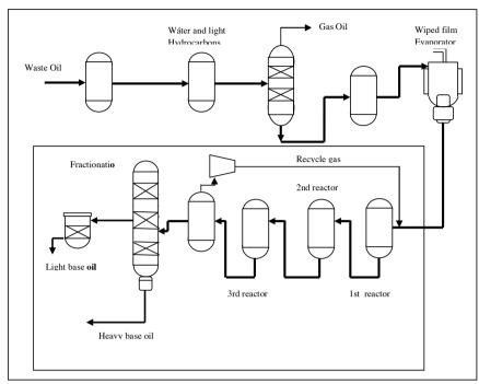
Figure 10 CEP simplfied process flow diagram source: CEP
