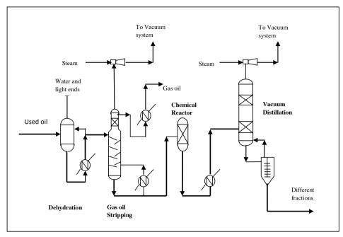
Figure 13 STP simplified process flow diagram Source STP
