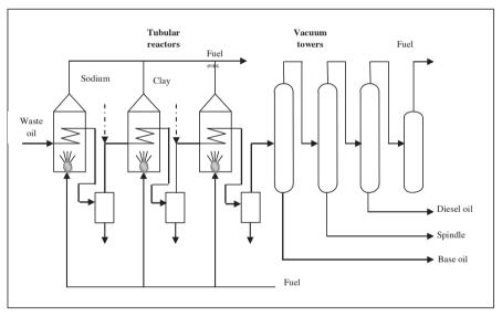
Figure 22 ENTRA simplified process flow diagram Source: Audibert (2006)
