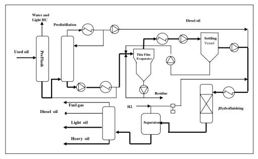
Figure 9 KTI simplified process flow diagram Source: Audibert as cited UNEP(2012)
