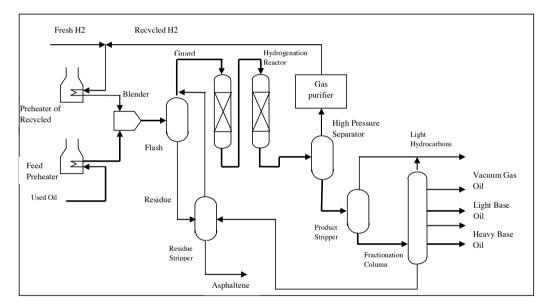
Figure 11 UOP Hylube simplified process flow diagram Source: UOP
