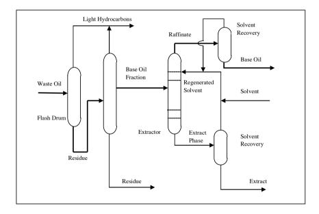
Figure 14 Probex simplified process flow diagram
